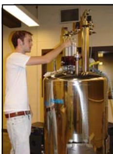
Tristan Gornall demonstrates Earlham's nuclear magnetic resonance (NMR) spectrometer, a key piece of equipment that is rare in most undergraduate laboratories.
